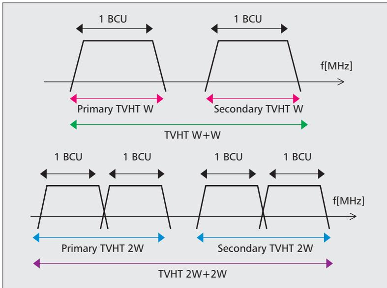
**Figure 3.** TVHT PHY channel configurations: TVHT  $W$ ,  $2W$ ,  $W+W$ , and  $2W+2W$
