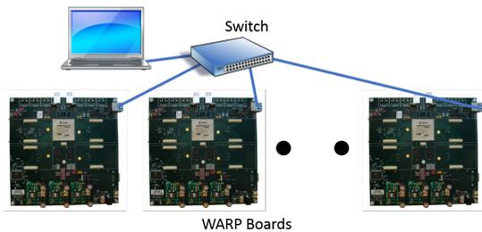
**Figure 2: The WARPLab design allows multiple WARP boards to be connected to and controlled by a single computer.**
