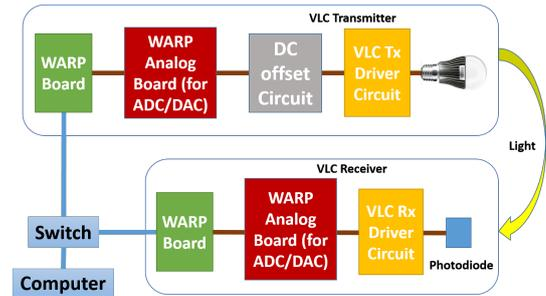
Figure 1: System architecture for a single Tx-Rx pair.
