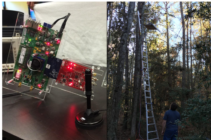
Fig. 4. Single-radio mobile node, omnidirectional antenna and outdoor installed AP.
