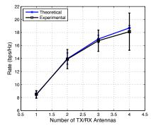
Fig. 3: Aggregate rate for a NLOS MxM system.
