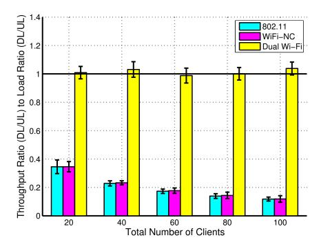
Figure 5.3: Mean throughput ratio (DL/UL) to load ratio (DL/UL) with symmetric load for different network densities.
