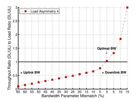
Figure 5.7: Impact of mismatch in optimal bandwidth setting on throughput to load ratio for asymmetric traffic.
