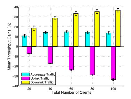
Figure 5.11: Dual Wi-Fi throughput gains over 802.11 with load asymmetry (DL/UL) of 4 for different network densities.
