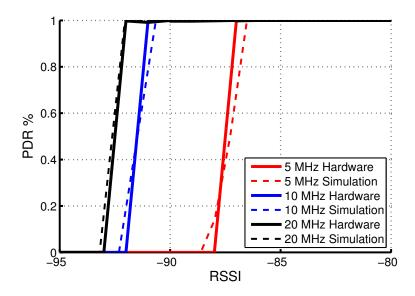
Figure 5.1: Packet Delivery Ratio (PDR) comparison between NS-2 simulation and commodity hardware.
