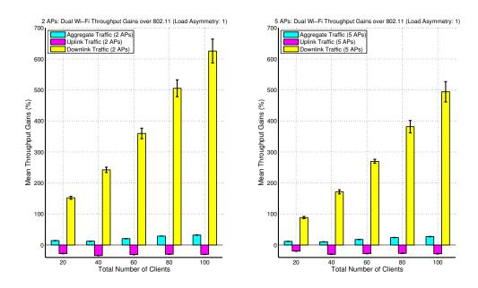
Figure 5.9: Dual Wi-Fi throughput gains over 802.11 with symmetric traffic. Left: 2 in-channel AP topology, right: 5 in-channel AP topology.
