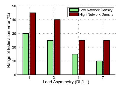
Figure 5.8: Range of bandwidth settings in which Dual Wi-Fi provides a closer ideal throughput ratio (DL/UL) to load ratio (DL/UL) than 802.11, as a fraction of the total bandwidth.
