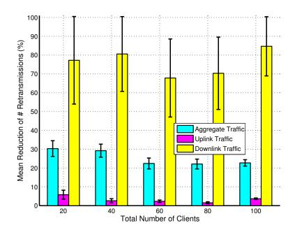
Figure 5.16: Average reduction of number of retransmissions per transmitted packet over 802.11 with symmetric traffic for topologies with 1-5 in-channel APs.
