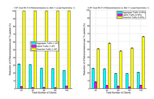
Figure 5.15: Mean reduction of number of retransmissions per transmitted packet over 802.11 with symmetric traffic. Left: 1 in-channel AP topology, right: 5 in-channel AP topology.
