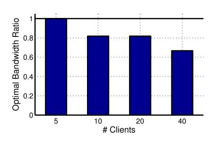
Figure 5.5: Dual Wi-Fi's optimal bandwidth ratio (DL/UL) based on network density for symmetric traffic.
