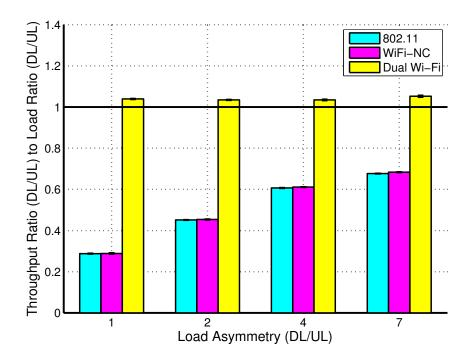
Figure 5.2: Proportion of throughput ratio (DL/UL) to load ratio (DL/UL) for 20 clients. Note that Dual Wi-Fi approximates ideal ratio (value of 1) for all load asymmetries.
