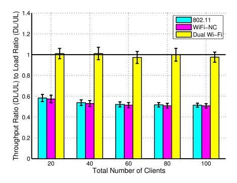
Figure 5.4: Mean throughput ratio (DL/UL) to load ratio (DL/UL) with load asymmetry (DL/UL) of 4 for different network densities.
