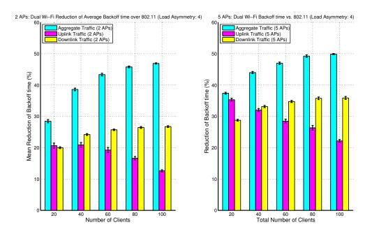
Figure 5.14: Mean reduction of backoff time per successful data transmission over 802.11 with load asymmetry (DL/UL) of 4. Left: 2 in-channel AP topology, right: 5 in-channel AP topology.
