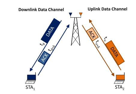
Figure 3.2: Bi-directional Data-ACK communication performed individually and asynchronously in each downlink and uplink data channels. Isolated downlink and uplink data channels, allow simultaneous transmissions even in clique networks.
