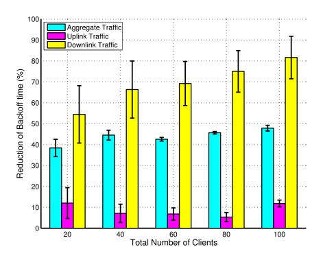
Figure 5.13: Mean reduction of backoff time per successful data transmission over 802.11 with symmetric traffic for topologies with 1-5 in-channel APs.
