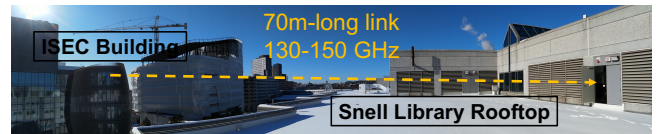
Figure 3: Outdoor backhaul-scale link above 100 GHz
